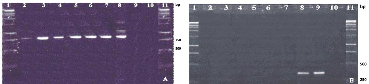
**Figure 1.** Molecular Identification of potato cyst-forming nematodes from Costa Rica with specific primers. A) *G. pallida* specific primers GpaF and GpaR. B) *G. rostochiensis* specific primers GroF and GroR. Lane 1, Molecular weight marker (M)= 1 kb (Fermentas); Lane 2, QLC11; Lane, QLC50a; Lane 4, QLC50b; Lane 5, QLC100; Lane 6, QPC100; Lane 7, *G. pallida*; Lane 8, *G. pallida* + *G. rostochiensis*; Lane 9, *G. rostochiensis*; Lane 10, Negative control; Lane 11, M= 1kb.
